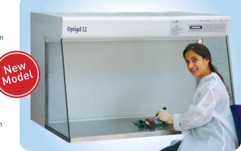
The new OPTIGEL provides a clean air working area of Class ISO-5, according to ISO-14644. Air is constantly blown horizontally through an absolute HEPA filter into the working area, thus protecting the product inside the cabinet from existing particles in the air.
